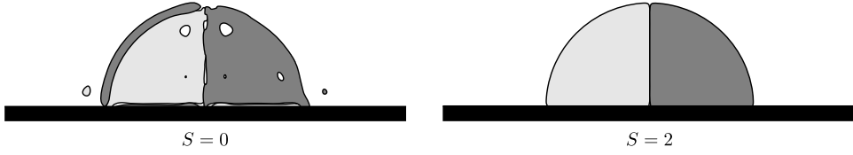
Fig. 5. Snapshots of compound droplets in contact with a flat substrate with respect to S = 0 and S = 2 .
